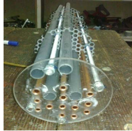
Fig. 1: Cross section of the hydro cooling system
